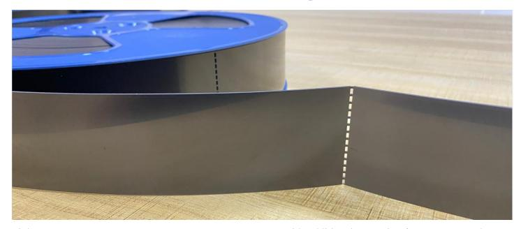
Sinho's SPECIAL PERFORATED SNAP REEL BANDS provide additional protection for components that are packaged in tape and reel. Sinho REEL BANDS are designed to wrap around the outer layer of carrier tape to resist the compressive forces that carrier tape alone can't withstand. The materials was perforated in every 1.09M long for 13" reels, every 1.25M long for 15" reels. All Reel Bands are composed of conductive polystyrene materials.
