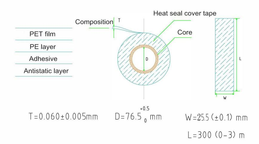
Name: Drawing for SHHT32D-25.5 HEAT SEAL COVER TAPE Wides also available for 5.4/9.3/13.3/21.3/37.5/49.5/65.5/81.5mm,(±0.1)mm
