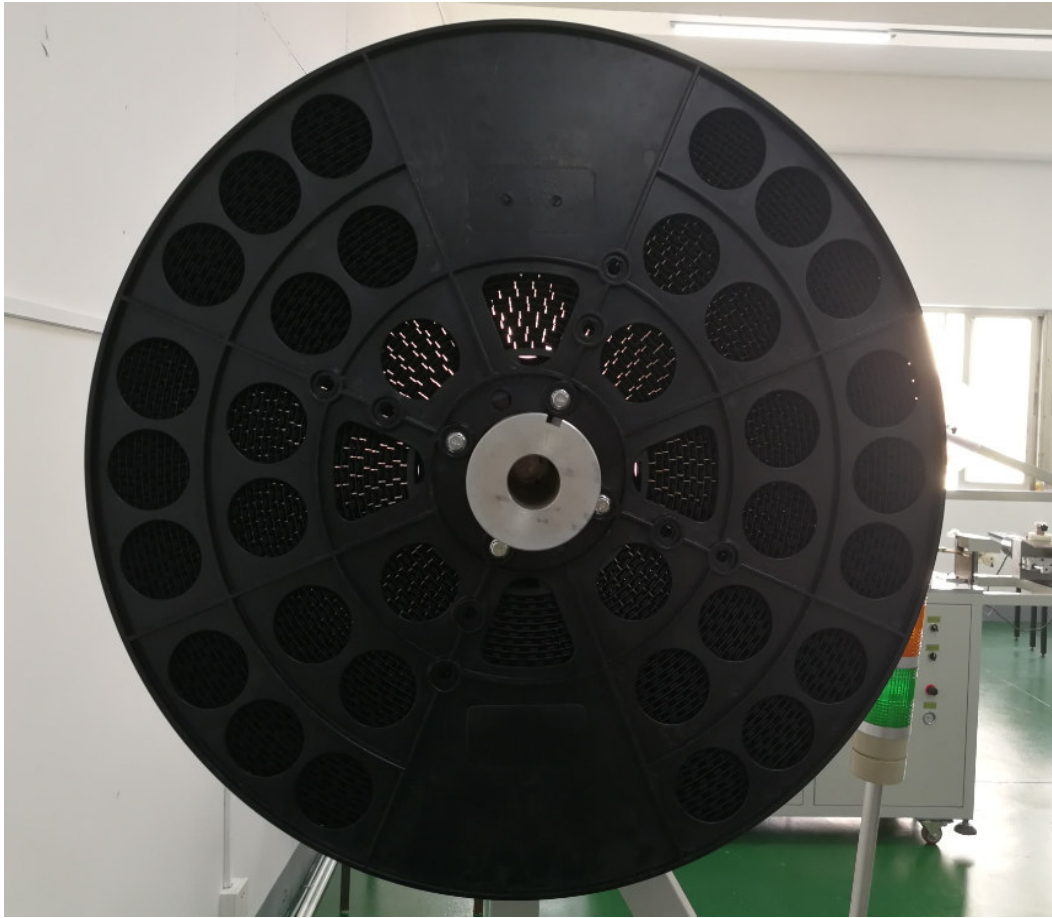
22" molded plastic reel with winding carrier tape on it
